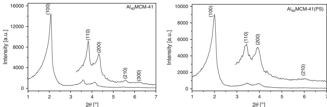
Fig. 1. Low-angle X-ray diffraction spectra of calcined samples. PS: post-synthesis.
