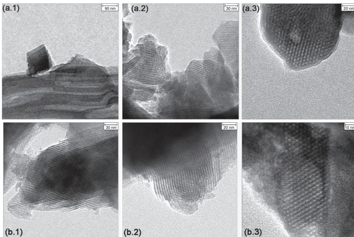
Fig. 3. Transmission electron microscopy image showing highly ordered, long-range hexagonal array of mesopores in  $\text{Al}_{40}\text{MCM-41}$  samples prepared by (a.1, a.2 and a.3) conventional, and (b.1, b.2 and b.3) post-synthesis alumination.
