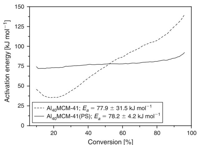
**Fig. 5.** Apparent activation energy for thermodesorption of the *n*-butylamine probe molecule on Al<sub>40</sub>MCM-41 samples prepared by conventional and post-synthesis (PS) alumination.
