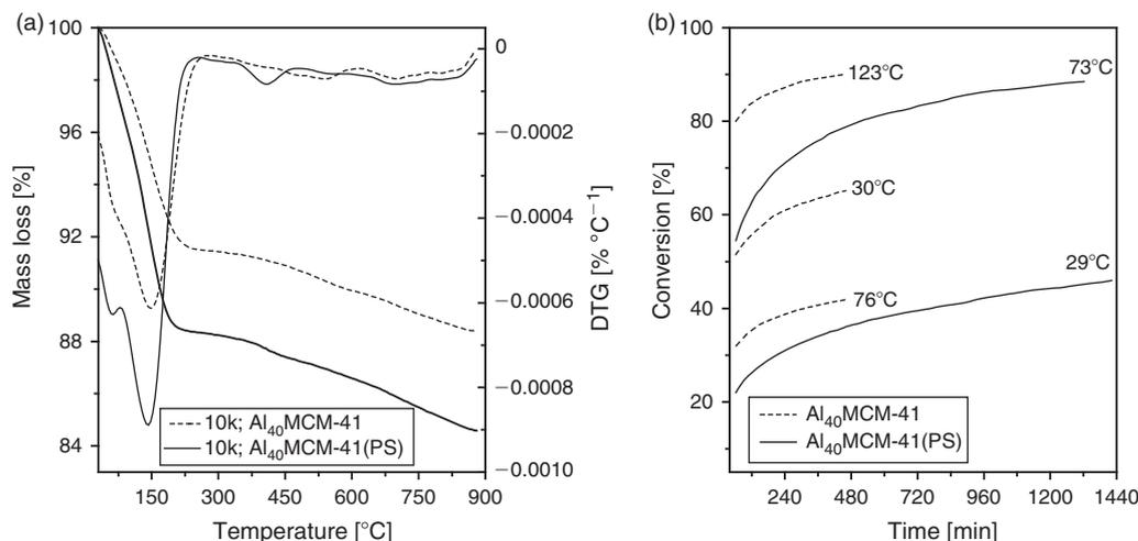
**Fig. 4.** (a) Thermogravimetric analysis/derivative thermogravimetric analysis curves, and (b) thermodesorption conversion of *n*-butylamine as a function of time at different temperatures for the Al<sub>40</sub>MCM-41 catalysts prepared by conventional and post-synthesis (PS) alumination (10k = heating rate of 10°C min<sup>-1</sup>).
