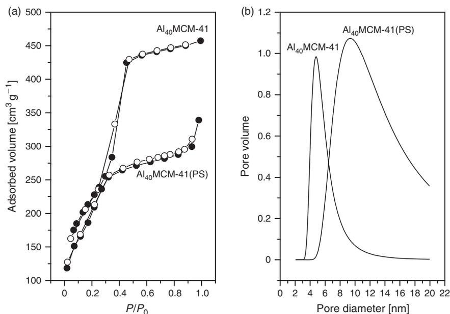
Fig. 2. Nitrogen adsorption isotherms and pore distributions of the  $\text{Al}_{40}\text{MCM-41}$  material prepared by conventional and post-synthesis (PS) alumination: (a) adsorption-desorption isotherms, and (b) pore size distribution (nm).
