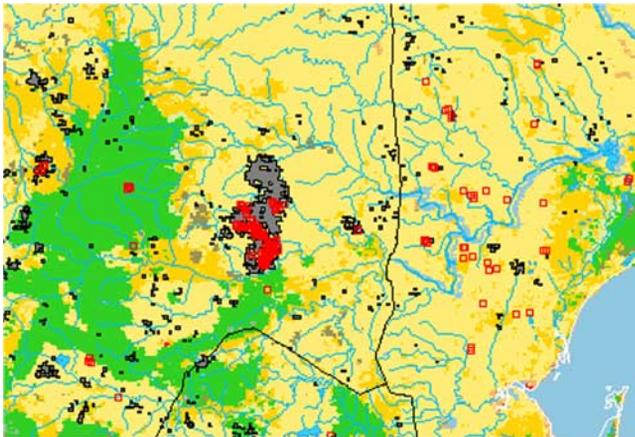
**Figure 3.** Example of results obtained using the ESA web map server (WMS) over the Kruger National Park, South Africa, in September 2000. The various layers displayed include the IGBP land cover classification, political boundaries and country borders, rivers and lakes (National Imagery and Mapping Agency), ATR-2 fires (red squares), and GLOBSCAR burnt areas (black polygons with shading).
