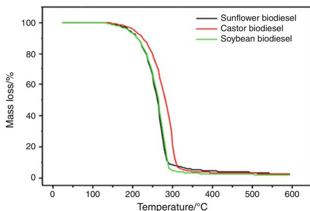
**Fig. 1** TG curves of the sunflower, castor, and soybean methylic biodiesel
