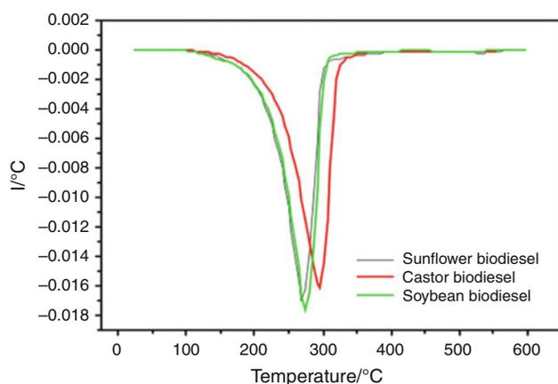
**Fig. 2** DTG curves of the sunflower, castor, and soybean methylic biodiesel
