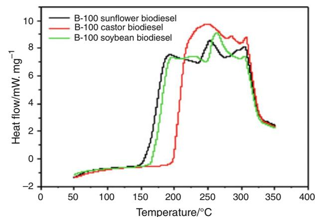
**Fig. 3** Profile PDSC curves for sunflower, castor, and soybean biodiesel obtained by dynamic method
